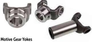
Yoke packages come complete with everything you need to install them in your vehicle, including: hardened grade-8 locknut, washer, and chromoly u-bolts. All Motive Gear billet chromoly yokes are 4120 or 4240H bar stock, computer-controlled heat treated to 34-38 Rockwell® C. All true billet yokes have the finest and most consistent quality hardened steel available.
